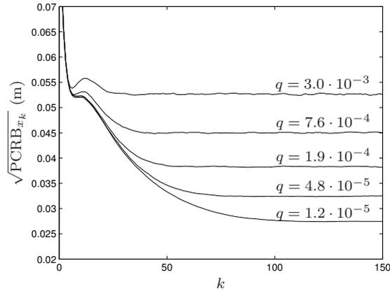
**Figure 4.** Example of square-root PCRb on estimation error for  $x_k$ , using the simplified observation model. Results obtained with a variable process noise parameter  $q$  (in  $\text{m}^2/\text{s}^2$ ) and  $P_S = 0.75$ .
