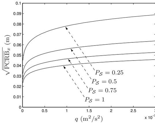
**Figure 6.** Steady-state square-root PCRB for  $x_k$  vs. process noise  $q$ , with variable probability parameter  $P_S$ .
