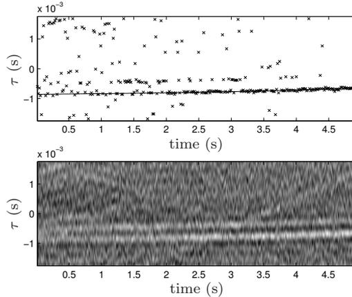
**Figure 1.** GCC results in reverberant environment, with fast-moving sound source (target speed approximately 1 m/s). *Bottom plot:* GCC output vs. time, dark areas represent low values. *Top plot:* the solid line indicates the target’s true time delay, ‘x’ markers denote the lags maximising the GCC output.
