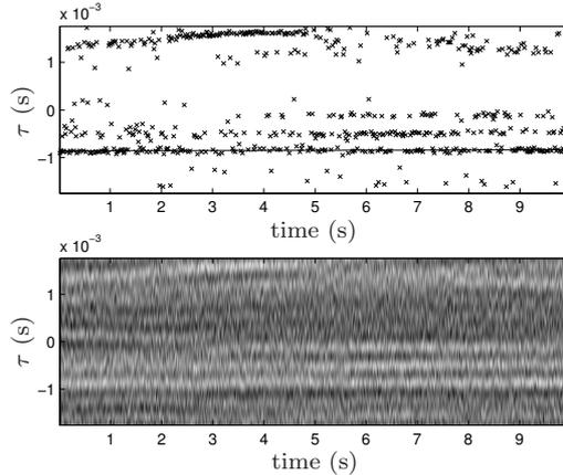
**Figure 2.** GCC results in reverberant environment, with slow-moving sound source (target speed approximately 0.1 m/s). *Bottom plot:* GCC output vs. time, dark areas represent low values. *Top plot:* the solid line indicates the target’s true time delay, ‘x’ markers denote the lags maximising the GCC output.
