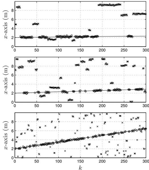
**Figure 8.** Realisations of the correlated observations process. Solid lines represent the target trajectory along the state space, ‘o’ markers denote observations for a correctly detected target, ‘x’ markers are erroneous observations. The source velocity  $\dot{x}_s$  is, from top to bottom, 0.05, 0.1 and 0.5 m/s. In all three cases, the detection probability is  $P_S = 0.5$ .
