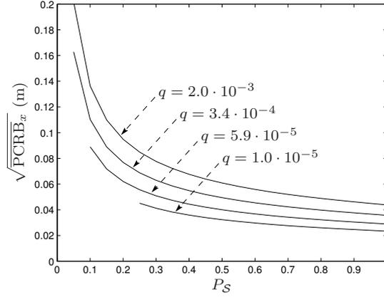
**Figure 5.** Steady-state square-root PCRB for  $x_k$  vs. target detection probability  $P_S$ , with variable process noise parameter  $q$  (in  $\text{m}^2/\text{s}^2$ ).
