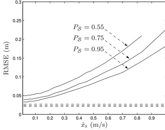
**Figure 10.** RMSE performance results for PF algorithm with simplified observation model. Dashed lines: PCRB results reproduced from Figure 9 (for corresponding values of  $P_S$ ).
