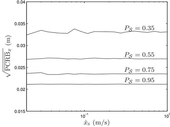
**Figure 9.** Steady-state square-root PCRB vs. target velocity  $\hat{x}_s$  computed for correlated observations, with variable detection probability  $P_S$ .
