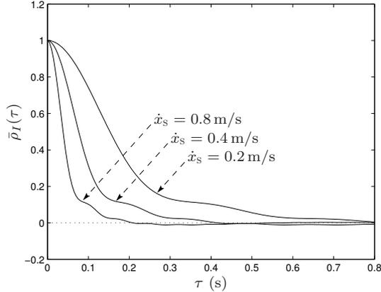
**Figure 7.** Temporal correlation coefficient for sound intensity, with variable target velocity  $\dot{x}_s$ .
