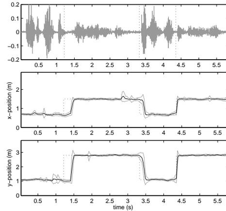
**Fig. 2.** *Top plot:* signal recorded with one array sensor. Vertical dotted lines denote a change of speaker. *Bottom plots:* tracking results in  $x$  and  $y$ -coordinates. Dotted lines represent the position of the active source.
