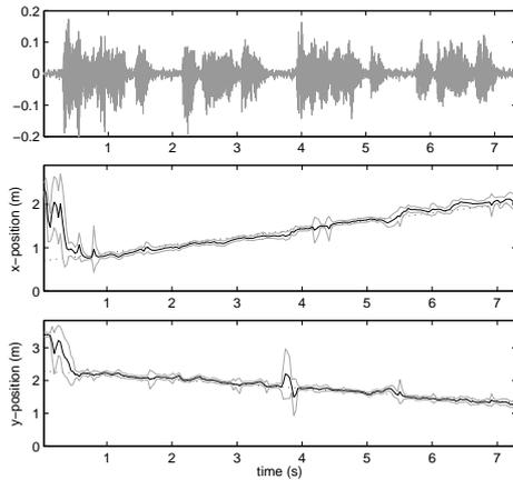
**Fig. 1.** *Top plot:* signal recorded with one array sensor. *Bottom plots:* true source position (dotted line), source location estimate (solid lines) and lines representing  $\pm$  one standard deviation of the particle set (grey lines).
